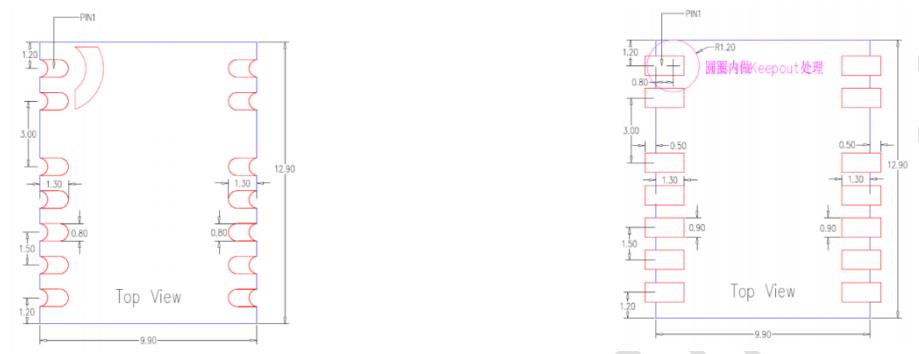
In order to facilitate the soldering of the stamp hole, the stamp hole pad needs to be extended by at least 0.5mm, so the package size of the module is recommended to be 12.9mm\*10.9mm\*2.3mm; Please go to Luat Technical Support Forum to download the module package:
