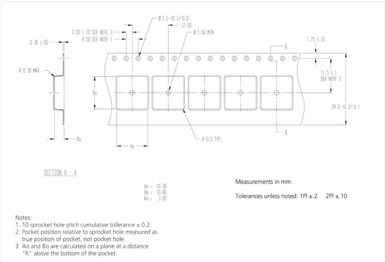
Figure 5: MAX-7 Tape dimensions
